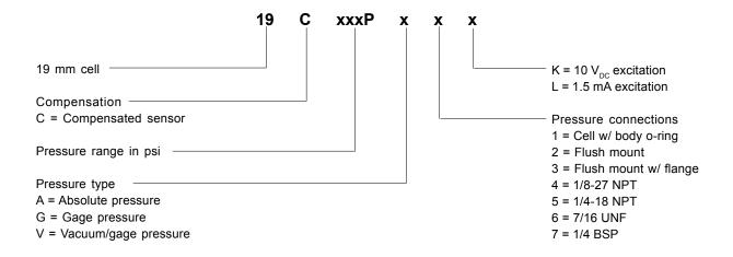
For example: part no. 19C100PA4K = 19 mm cell, compensated, 100 psi, absolute, 1/8NPT port, with 10  $V_{DC}$  excitation
