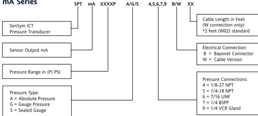
For example: Part #**SPTmA0100PA4W02** = SPT mA Sensor, 100 psi, Absolute, 1/8NPT Port with a 2 feet cable (pigtail) electrical connection.
