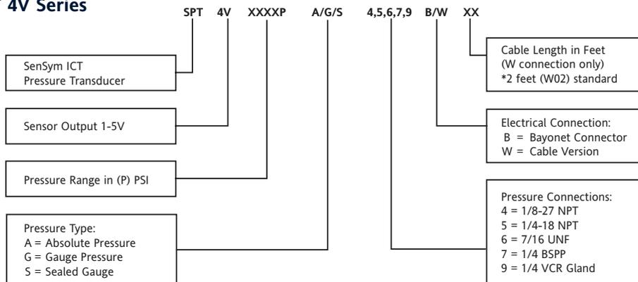
For example: Part #**SPT4V0100PA4W02** = SPT 4V Sensor, 100 psi, Absolute, 1/8NPT Port with a 2 feet cable (pigtail) electrical connection.
