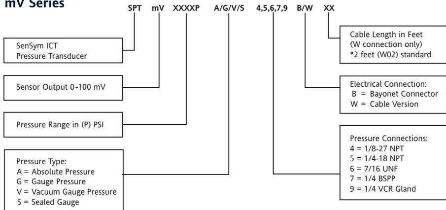
For example: Part #**SPTmV0100PA4W02** = SPT mV Sensor, 100 psi, Absolute, 1/8NPT Port with a 2 feet cable (pigtail) electrical connection.
