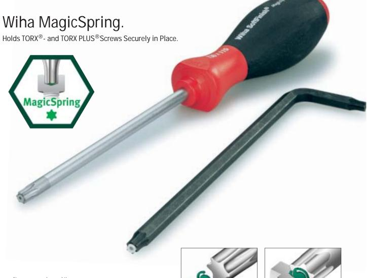
No more annoying and time-consuming hunting around for TORX® or TORX PLUS® screws that have apparently vanished into thin air. With Wiha's ingenious new tool, the MagicSpring, TORX® or TORX PLUS® screws\* are kept firmly where you want them. The highlight of the "MagicSpring" tools is the stainless steel "magical" retaining spring that, together with a thin cover disc, is laser-welded to the tip of the blade.
