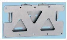
Wall mounts designed for medium sized LCD screens that have a VESA MIS-E mounting pattern of 200mm x 100mm. They can also be used to mount screens with VESA MIS-D 100mm x 100mm. Maximum weight of screen is 24kg.
