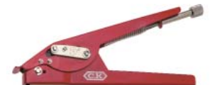
▲ 50020 TIE GUN FOR CABLE BINDER 220 mm 8.3/4" Strong stainless steel body, red lacquered. Pulling force adjustable. Cuts automatically as soon as the requested pulling force has been reached. For cable binder width 4.7 - 13 mm (.185 - .512").
