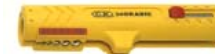
▲ 30150 CABLE WIRE STRIPPER 8 - 13 mm 5/16 - 1/2" Ø C.K.-Jokari Cable Stripper (No. 15) with additional precision wire stripping blades, retractable safety trimming knife blade, splicing blade, pocket clip. For easy and quick stripping of sheathing of round cable from 8 - 13 mm (5/16 - 1/2") Ø. For stripping of solid and stranded conductors of 0.2, 0.3, 0.8, 1.5, 2.5, 4.0 mm 2 (24, 22, 20, 16, 14, 12 AWG). No adjustment necessary. Also for use in very confined spaces, e.g. junction boxes, switch consoles etc.
