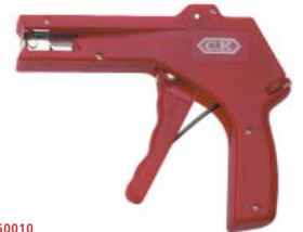
▲ 50010 TIE GUN FOR CABLE BINDER 165 mm 6.1/2" Fibre glass reinforced plastic body, light, yet strong. Pulling force adjustable. Cuts automatically as soon as the requested pulling force has been reached. For cable binder width 2.4 - 4.8 mm (.094 - .189").
