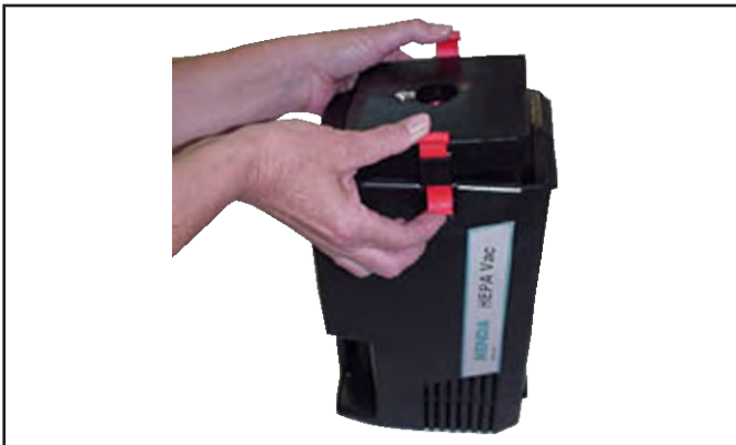
Figure 3: Lifting out the cartridge.
