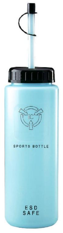
32-oz. static dissipative sports bottle for personal consumption of cold drinks. These bottles offer an average surface resistivity of  $10^9$  to  $10^{10}\Omega$  and can dissipate a  $\pm 5000$ V charge of in less than 2 seconds at 40% relative humidity.
