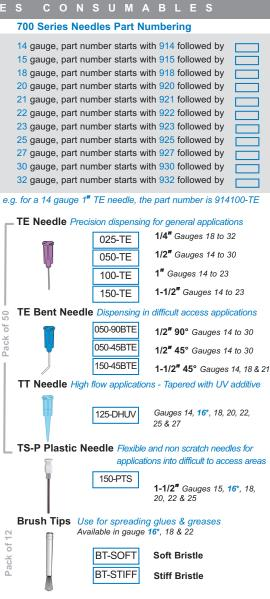
16\* : Only the TT, TS-P and Brush Tips are available in 16 gauge For ordering, the part number starts with 916
