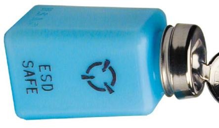
pump with air tight check valve. Features an average surface resistivity of  $10^9 \sim 10^{10}$  ohm, and can dissipate a  $\pm 5000V$ Static dissipative dispensers come with a stainless steel charge in less than 2 seconds at 40% relative humidity.
