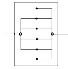
Terminals 1 and 6 are frequently unused, 2 pair (4 wire) cable is normally used in these installations. All wiring in parallel, i.e. terminal 1 on master socket to terminal on secondary socket, terminal 2 to terminal 2, etc.
