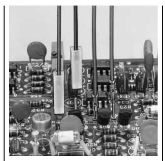
This small single-circuit connector connects to 1.0mm (.039") and 1.3mm (.051") diameter pins and requires only minimal space for connection of wires to high-density printed circuit boards. The SMF connector has a funnel shaped lead-in to ease insertion and to ensure a balance with its high retaining force.
