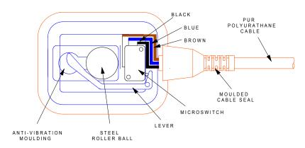
The micro-switch assembly inside the float, axially mounted in line with the weight, changes contacts according to the float's position, as in the diagram below. Therefore as the liquid level drops or rises slowly, a pump or flow control suitably connected, can be switched in or out to maintain an average level of the liquid. By connecting only one side of the switch, the unit can be also used to fill or empty the tank as required.
