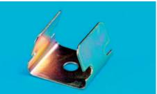
It is a requirement of BS5839 Part 1 that surface mounted Fire Performance cables must be secured using metallic fixings that can withstand the same temperatures and vibration as the Fire Performance cables.
