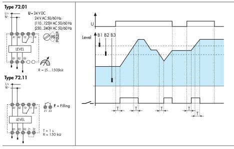
**Filling Control** – between Min. and Max. levels.
