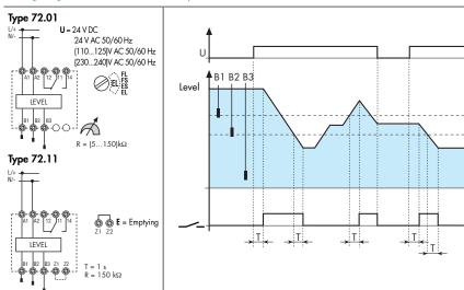
Emptying Control - between Max. and Min. levels. Under normal operation the liquid level can be expected to cycle between the Maximum and the Minimum electrodes, B1 and B2 (plus a degree of over and under-shoot).
