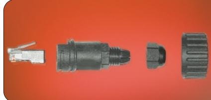
between each connection point. The RJ-Lnxx<sup>®</sup> field attachable connector enables bulk cable to be pulled to the exact required length, and then terminated to the RJ-45 plug using readily available crimp tools. The completed assembly provides the same sealed, robust connector as the RJ-Lnxx overmolded cordset.
