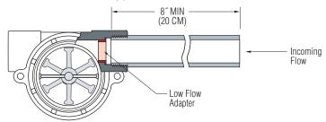
Except for straight-thread versions, RotorFlow sensors connect to piping via NPT mating thread forms. The use of an appropriate thread sealant is necessary to assure a leak-tight connection. Permatex "No More Leaks®" or 2 wraps of Teflon® tape are the only sealants recommended for GEMS flow sensors. Straight-thread versions require an 0-ring for sealing.
