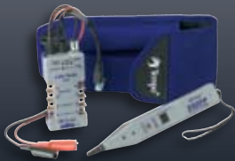
NEW 802K Digital LAN Tracing Kit
