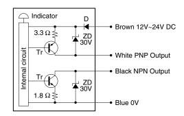
Upon overload or short circuiting, the output transistor turns off. Power up again after removing the cause of the overload/short circuit.
