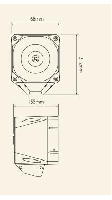
The Asserta Industrial warning sounder / beacon is designed to cope with harsh environments requiring protection to IP66. Design features are incorporated to ensure safer and easier installation, while providing flexibility with fewer product variants.
