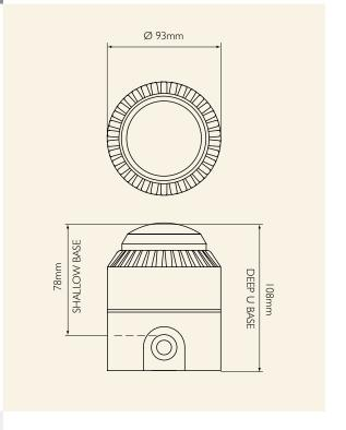
The use of beacons to supplement audible alarms is becoming increasingly common. A combined sounder beacon allows both an audible and visual alarm to be provided but requires only a single installation point. LED beacons have a dramatically lower current consumption than that of traditional xenon beacons making them ideal for applications where sounder circuit capacity is limited.
