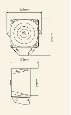
The Asserta Midi Sounder Beacon is a versatile and rugged audio-visual alarm designed for industrial environments or areas where there is a requirement for a physically robust and well-protected unit. A range of supply options permit use with a wide range of fire and process systems.
