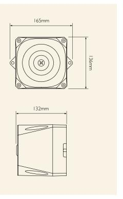
The Asserta Midi Sounder is versatile, compact unit that has been designed for industrial environments or areas where there is a requirement for a physically robust and well protected alarm is required. A range of supply options permit use with a wide range of fire and process systems.
