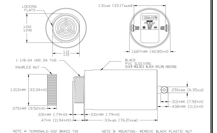
AND INSERT THREADED FRONT THROUGH 1.25" HOLE PUNCHED IN PANEL, IF ORIENTATION IS NEEDED, NOTE LOCKING
