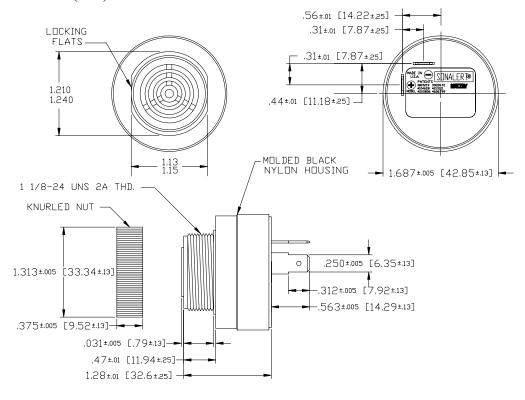
NOTE A: TERMINALS-.032 BRASS, TIN PLATED WITH .070 DIA. WIRE HOLE. WILL ACCEPT 1/4" QUICK CONNECT.
