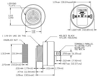
NOTE A: TERMINALS-032 BRASS TIN PLATED, TAPPED FOR #6-32 SCREW. TWO #6-32 NICKEL PLATED BRASS SCREWS INCLUED. WILL ACCEPT 1/4\* QUICK CONNECT. NOTE B: MOUNTING- REMOVE BLACK PLASTIC NUT AND INSERT THREADED FRONT THROUGH 1.25' HOLE PUNCHED IN PANEL, IF ORIENTATION IS NEDED, NOTE LOCKING FLATS ON DRAWING. SCREW NUT BACK ON. DO NOT OVERTIGHTEN.
