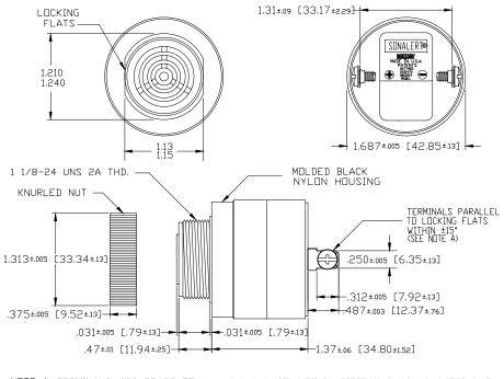
NOTE B: MOUNTING- REMOVE BLACK PLASTIC NUT AND INSERT THREADED FRONT THROUGH 1.25" HOLE PUNCHED IN PANEL, IF ORIENTATION IS NEEDED, NOTE LOCKING FLATS ON DRAWING. SCREW NUT BACK ON. DO NOT OVERTIGHTEN.
