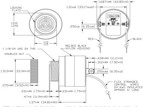
The red and black leads control the several functions. A logic 'Low' is a voltage less than 1/3 of supply voltage. A logic 'High' is a voltage greater than 1/2 supply voltage. A red or black input lead left unconnected is considered an open state.
