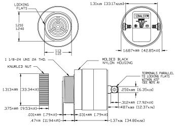
NOTE A: TERMINALS-032 BRASS TIN PLATED, TAPPED FOR #6-32 SCREW. TWO #6-32 NICKEL PLATED BRASS SCREWS INCLUBED. WILL ACCEPT 1/4' QUICK CONNECT. NOTE B: MOUNTING- REMOVE BLACK PLASTIC NUT AND INSERT THREADED FRONT THROUGH 1.25' HOLE PUNCHED IN PANEL, IF DRIENTATION IS NEEDED, NOTE LOCKING FLATS ON DRAWING. SCREW NUT BACK ON. DO NOT DVERTIGHTEN.
