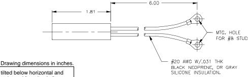
Tilt switches "make" when the electrode is tilted below horizontal and "break" when tilted above the horizontal. Total travel from "make" to "break" is the "Maximum included angle" shown below. The component to which the switch is attached must have a total tilt angle greater than the "Maximum included angle" for proper operation.
