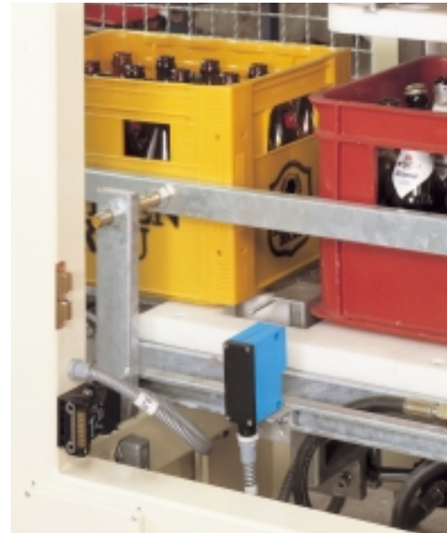
◀ WL 36 photoelectric reflex switches checking the presence of beer crates before automatic removal of the bottle caps.
