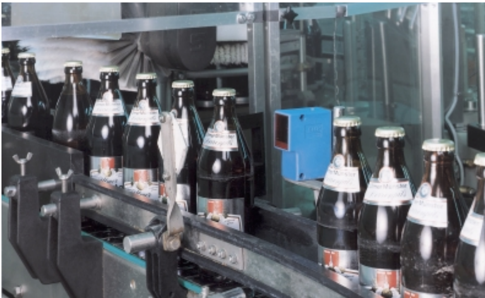
◀ Making sure that crates are full: WL 36 photoelectric reflex switches used to count coloured bottles before packaging.
