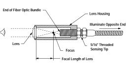
Lenses are most efficient when they are located slightly beyond their focal length distance from the sensing end of the fiber optic bundle. The easiest way to focus a lens is to treat it like a magnifying glass.
