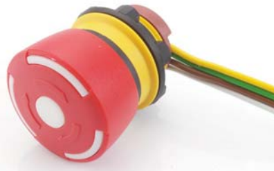
Emergency-stop non illuminated, ribbon cable, twist release, 32mm diameter for 22.5mm mounting, foolproof to EN 60947-5-5
