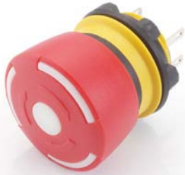
Emergency-stop non illuminated, plug-in terminals, twist release, 32mm diameter for 22.5mm mounting, foolproof to EN 60947-5-5
