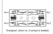
If the No. 3 contact welds. Each of the three form "a" contacts (No. 1, 2, and 4) maintain a gap of greater than 0.5 mm .020 inch.
