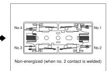
If the No. 2 contact welds. The single form "b" contact (No. 3) maintains a gap of greater than 0.5 mm .020 inch.
