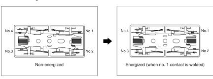
If the No. 1 contact welds. A gap of greater than 0.5 mm .020 inch is maintained at each of the two form "a" contacts (No. 2 and 4).
