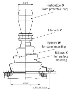
1) Panel cutout for assembly with bellows **W**
