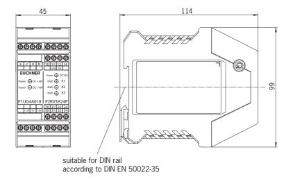
The universal power supply unit P1/P2 comprises the unit P1UG4A018 (P1) for the supply of the EUCHNER series KP joystick.
