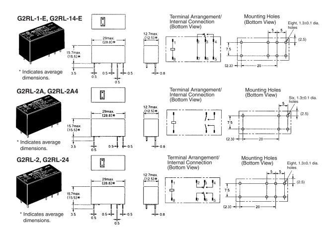
**ALL DIMENSIONS SHOWN ARE IN MILLIMETERS.**To convert millimeters into inches, multiply by 0.03937. To convert grams into ounces, multiply by 0.03527.
