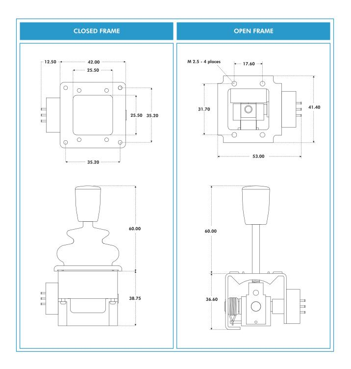
Note: The dimensions shown are for a generic two axes 4000 Series open frame with the E type handle, and a generic two axes 4000 Series closed frame also with the two axes E type handle. For specific dimensions of this or any other configuration please refer to Apem.
