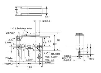
Simulated Hinge Lever SSG-01L3P SSG-5L3P SSG-01L3P-5 SSG-51L3P-5
