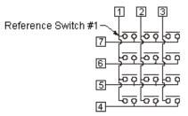
X - Y matrix output circuit configuration switch function - SPST NO momentary.
