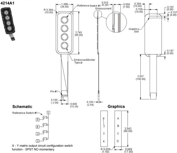
Both inserts supplied with each keypad Dimensions : Inches (Millimetres)
