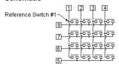
X - Y matrix output circuit configuration switch function - SPST NO momentary.
