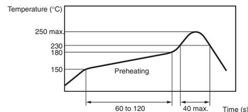
Do not use reflow soldering for any models other than the A6S-H and A6H. Otherwise the plastic case may melt or deform.
