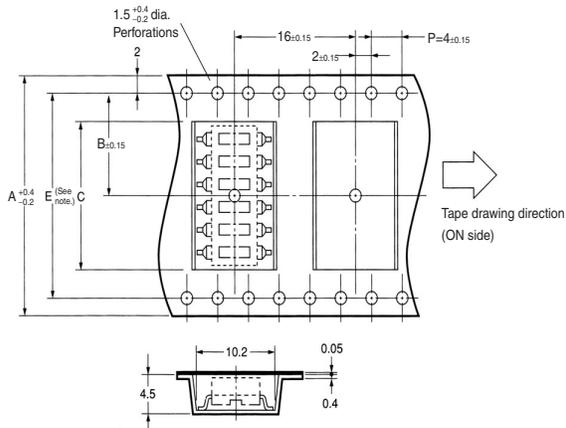
**Note:** The perforations along both sides are for Switches with 7 poles or more. The perforations on the bottom of the diagram are not provided on Switches with 6 poles or less.
