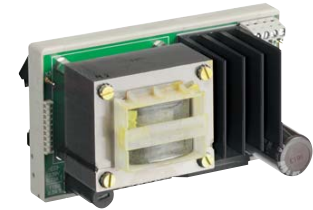
Power supply unit 24 V / 1 A regulated
