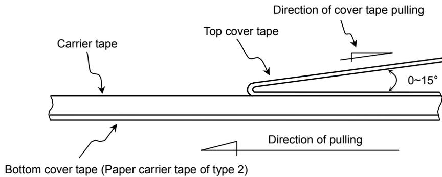
3-2. Carrier tape shall be flexible enough to be wound around a minimum radius of 30mm with components in tape.
