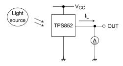
Note 5: Switching time measurement method
