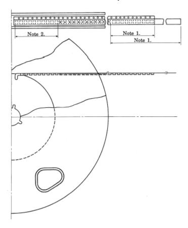
Note 1: The leader portion shell consist of cover tape minimum length of 300 mm and a piece of carrier tape with empty portion of 100 mm minimum.
