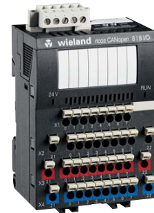
Compact modules CANopen CE; Approvals: in preparation
