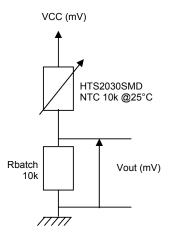
$$V_{OUT}(mV) = \frac{Vcc(mV) * R_{batch}(\Omega)}{R_{batch}(\Omega) + NTC_{HTS 2030 SMD}(\Omega)}$$
