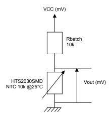
$$V_{OUT}(mV) = \frac{V_{CC}(mV) * NTC_{HTS 2030 SMD}(\Omega)}{R_{batch}(\Omega) + NTC_{HTS 2030 SMD}(\Omega)}$$
