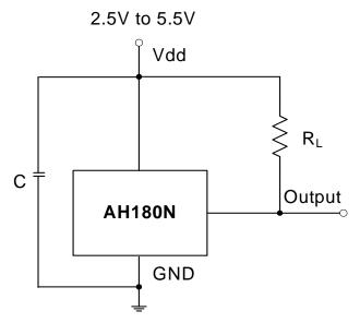
Note: C is for power stabilization and to strengthen the noise immunity, the recommended capacitance is  $10nF \sim 100nF$ . R<sub>L</sub> is the pull-up resistor, the recommended resistance is  $10kOhm \sim 100kOhm$ .
