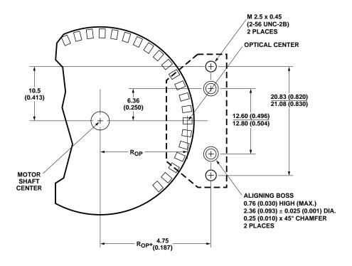
Figure 2. Mounting plane side B.
