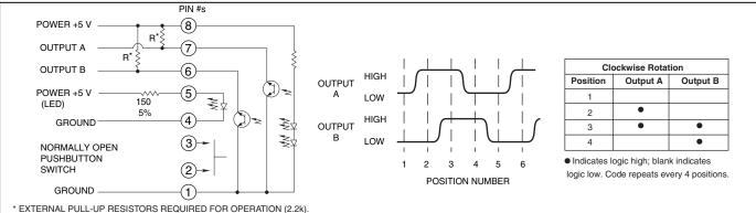
\*\* Circuit shown with on-board lighting system. Versions without on-board lighting system do not have LED power connections. Refer to standard 62A series for circuitry.
