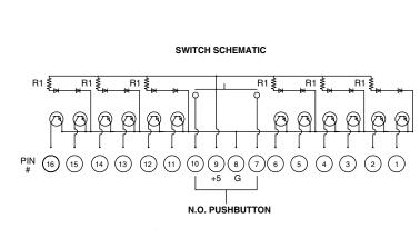
Note: External pull-up resistors required for operation. 20ký is suggested.
