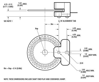
ALL DIMENSIONS FOR MOUNTING THE MODULE/CODESTRIP SHOULD BE MEASURED WITH RESPECT TO THE TWO MOUNTING POSTS, SHOWN ABOVE.
