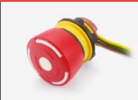
Emergency-stop non illuminated, ribbon cable, twist release, 32 mm diameter for 22.5 mm mounting, foolproof to EN 60947-5-5
