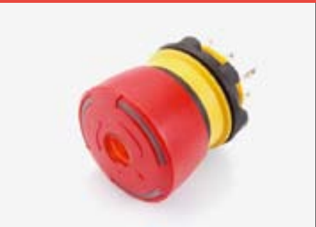
Emergency-stop red LED illuminated, plug-in terminals, twist release, 32 mm diameter for 22.5 mm mounting, foolproof to EN 60947-5-5
