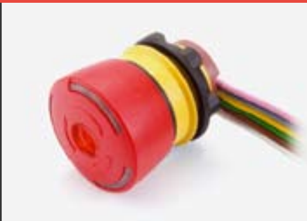
Emergency-stop red LED illuminated, ribbon cable, twist release, 32 mm diameter for 22.5 mm mounting, foolproof to EN 60947-5-5
